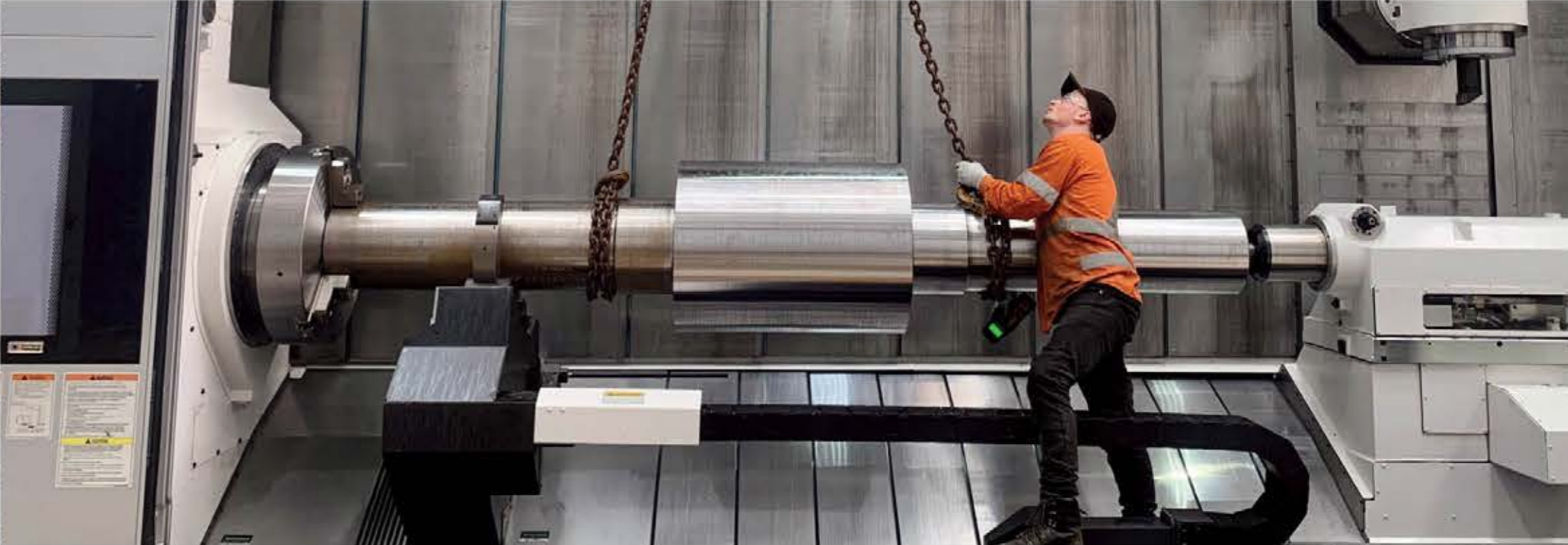
4,000kg Pinion Shaft, locally forged, locally machined (above and below)
