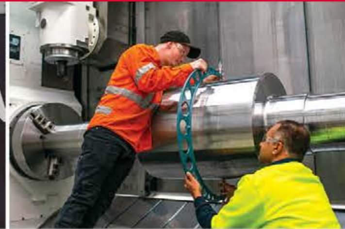
4,000kg Pinion Shaft, locally forged, locally machined (above and below)
